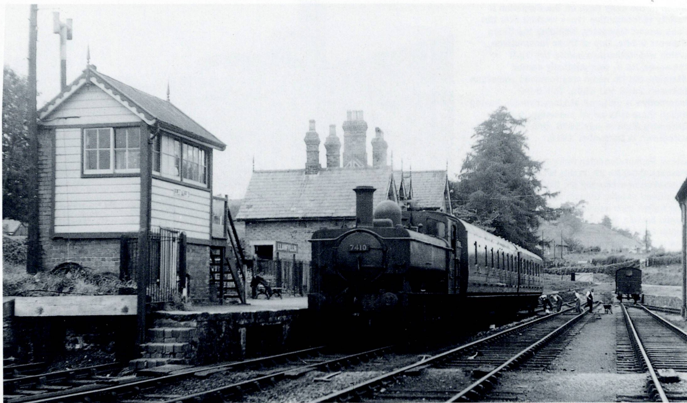
Above: Waiting to depart from the Llanfyllin terminus with the 1.25pm train for Oswestry on 14 September 1956, Collett 0-6-0PT No 7410 is pictured with the customary 2-coach 'B Set' used at that time on the branch line's passenger services, incorporating vehicles Nos 6773 and 6774. The train stands at the single 385ft-long platform with its brick & timber signalbox. It appears that some form of track maintenance is taking place in the station area. R. M. Casserley
